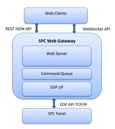
The SPC Web Gateway communicates (southbound) to the SPC panel over network using Siemens EDP protocol and offers a northbound interface - referred as Web Server - used by applications or web pages - referred as Web Clients - to operate and get information from the SPC panel. A REST JSON API is used for requests and commands and a WebSocket API for sending SIA events to the Web Clients.
